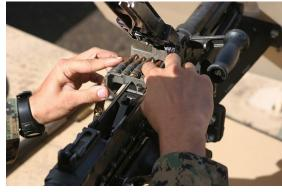
Feed Tray/Feed Tray Cover - Component that holds and guides ammunition (see top right photo)
